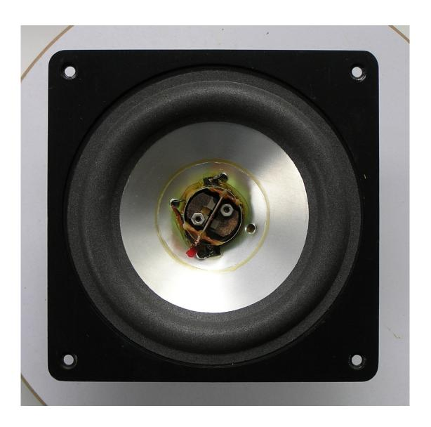
Apply a few drops of thinner onto the cone, so that the glue that holds the dustcap is moistened. Use a sharp knife and circle round and round on the bond until it comes off. Above you can clearly see the feedback system when the cap is removed.
